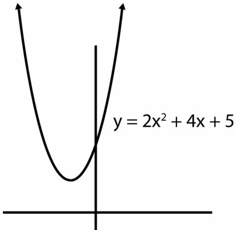
*There is no point on the graph where  $y$  is zero. So there is no solution to  $0 = 2x^2 + 4x + 5$  in the real numbers. If we extend our possibilities to the complex numbers, we see there are two complex numbers that make the equation  $0 = 2x^2 + 4x + 5$  true. The QUADRATIC (or QUAD2) program tells us that the two complex solutions are  $x = -1 \pm 1.22i$ .*
