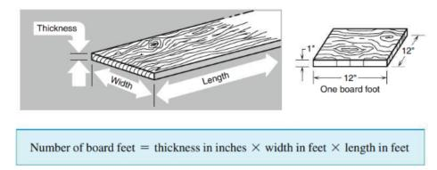
To find the number of board feet in a piece of lumber, multiply the length in feet by the width in feet by the thickness in inches. A thickness of less than 1 in. should be counted as 1 in. If the lumber is dressed or finished, use the full size or rough stock dimension to calculate board feet.
